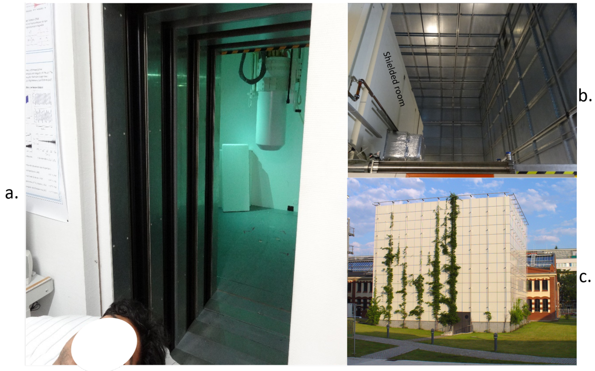
Figure 3.2: The MCG measurement room in PTB Berlin facility. a. The gate of the shielded room. b. The space outside the shielded room and the active shielding surrounding it. c. The active shielding layer from outside.
