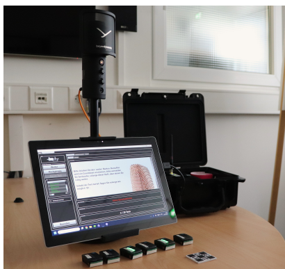
Figure 2: Measurement setup including the microphone, tablet and Delsys Trigno Avanti surface EMG sensor system.
