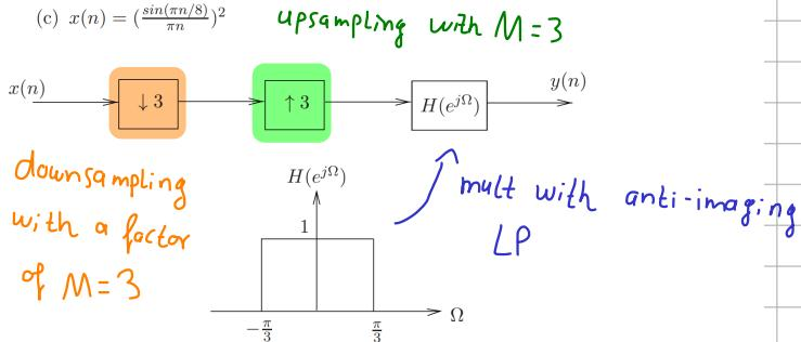
**Downsampling:** Re-sample a signal  $x(n)$  that has a sampling rate of  $f_s$
