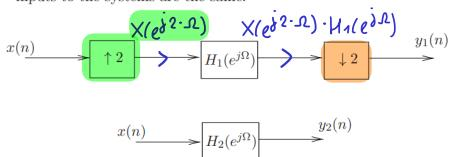
$y_1(e^{j\Omega})$  is  $X(e^{j2\cdot\Omega}) \cdot H_1(e^{j\Omega})$  downsampled by  $M=2$
