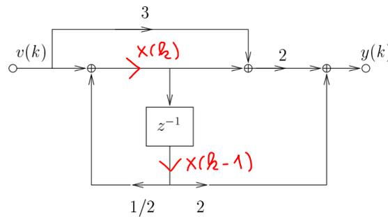
Figure 1: Signal flow graph of a filter
