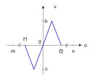
(f) The signal x(n) is to be amplitude modulated. Write down the modulation equation (2 P) in general terms. The carrier signal should also be transmitted.
